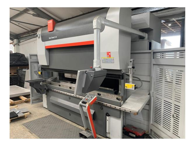
Hydraulic 2 cylinder downstroking press brake with Bystronic touch screen CNC Control.
