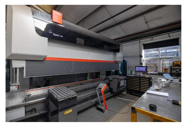
Hydraulic 2 cylinder downstroking press brake with Bystronic touch screen CNC Control.
